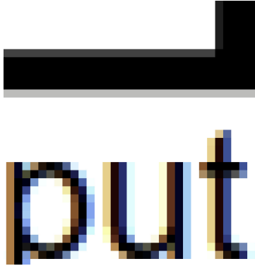
Figure 3.7: Aliasing typically found near hard edges to increase the apparent resolution or contrast. The shade of gray is not the same on both sides of the edge.
